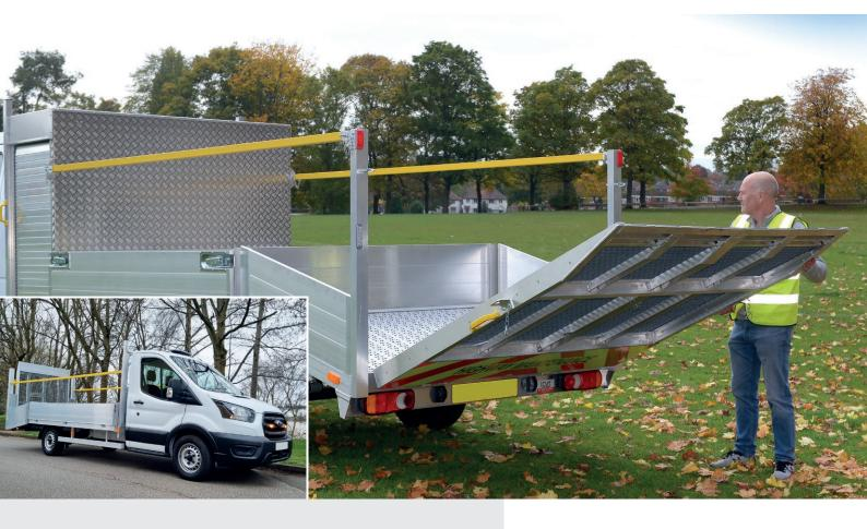
Payload of the vehicle was crucial to allow it to carry the majority of commercial mowers, and waste material over the winter period. Dependant on the chosen donor chassis cab, payload is as high as 1,280kg
