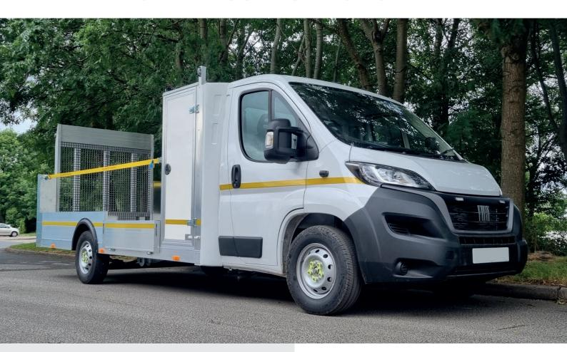
The vehicle is available in varies lengths depending on the final application and offers up to 1,500kg of payload dependent on the options fitted and body length. The internal width between the wheel boxes can be up to 1,800mm allowing the widest commercial mower to be carried.
